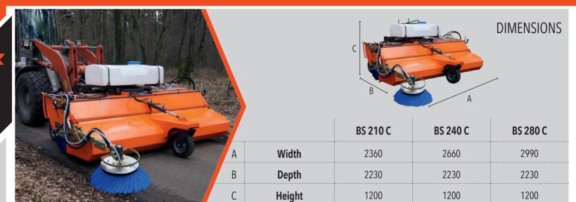
The Sweeper Bucket M3 series C is suitable for the cleaning of pavings and courtyard areas of industrial plants.
